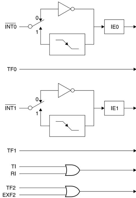
The Timer 0 and Timer 1 flags, TF0 and TF1, are set at S5P2 of the cycle in which the timers overflow. The values are then polled by the circuitry in the next cycle. However, the Timer 2 flag, TF2, is set at S2P2 and is polled in the same cycle in which the timer overflows. For further information, see the Microcontroller Data Book, section titled "Interrupts."
