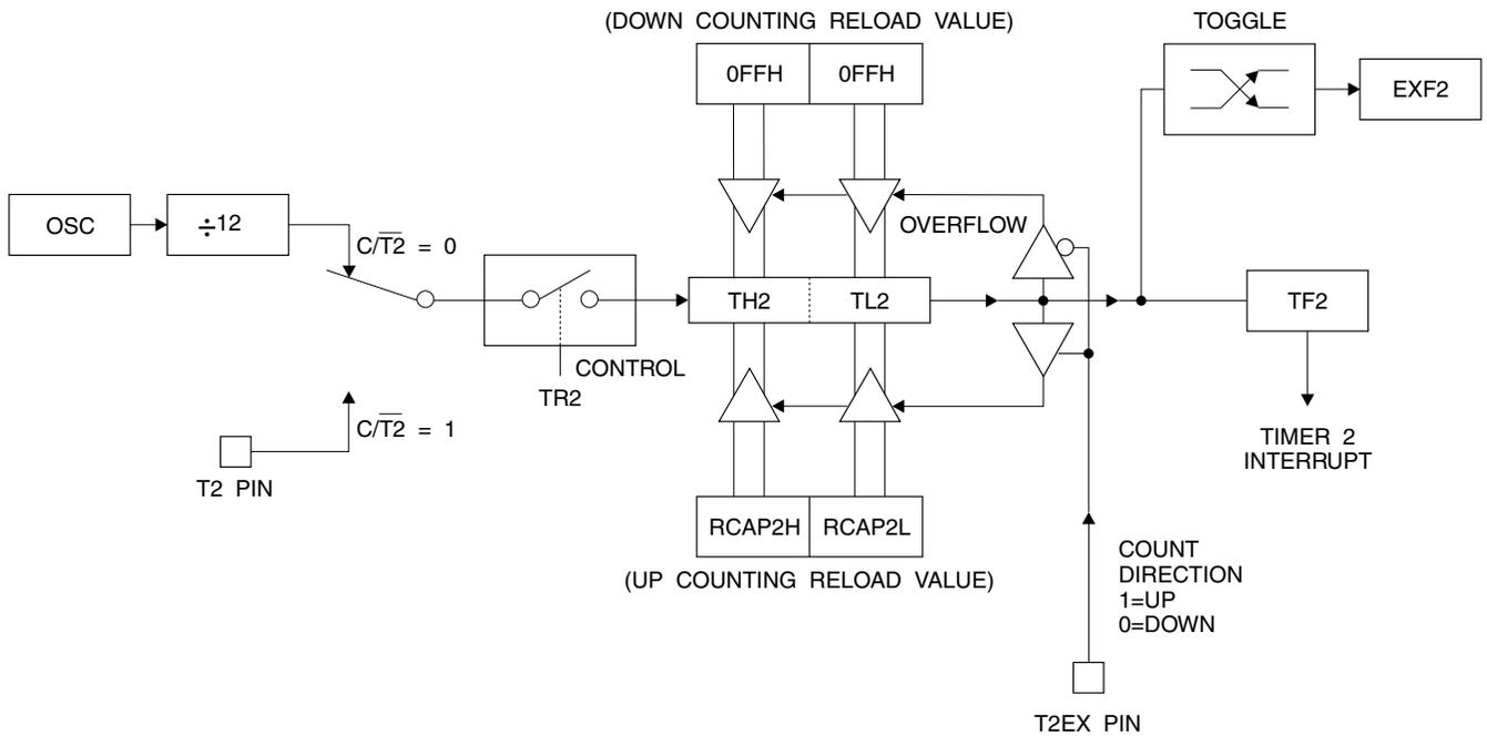
**Figure 4. Timer 2 in Baud Rate Generator Mode**
