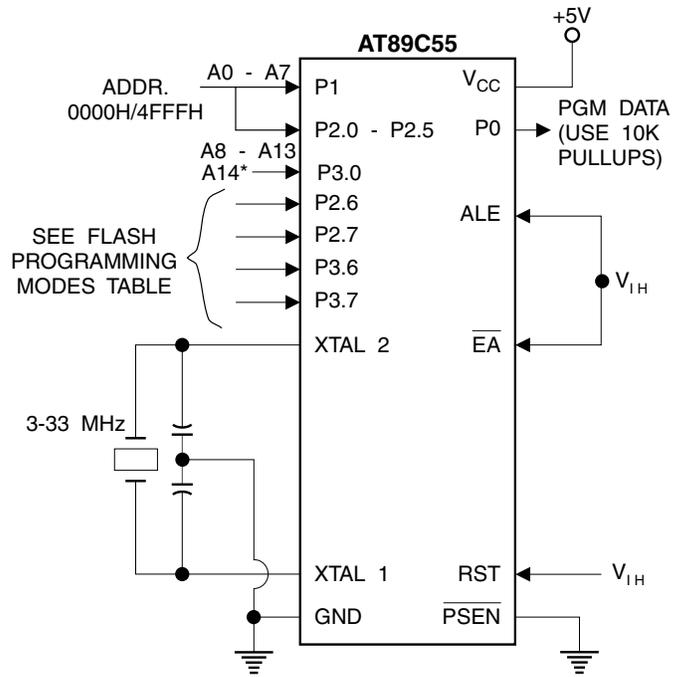
Note: \*Programming address line A14 (P3.0) is not the same as the external memory address line A14 (P2.6)
