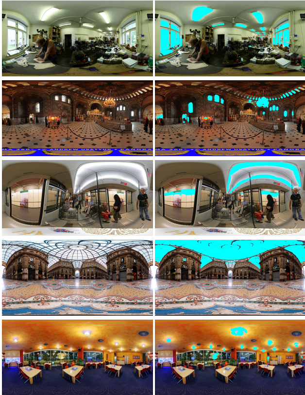
Fig. 5. Light detection results on SUN360 panoramas. (left) the input LDR panoramas; (right) light detection results, shown in cyan and overlaid on the original panorama for reference. The detector is able to handle a wide range of lighting arrangements, including large light patches and spotlights.
