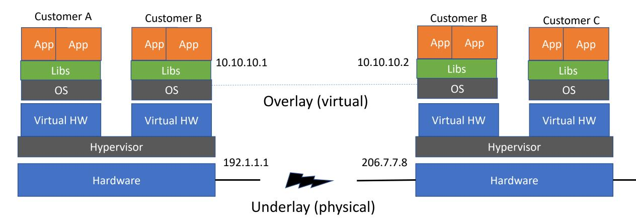
Forwarding between VMs involves a DNS-style lookup from overlay address to underlay location
