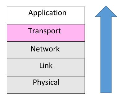
Transport layer provides end-to-end connectivity across the network
