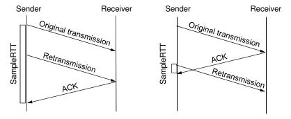
• Solution: Don't measure RTT for retransmitted packets and do not relax backed of timeout until valid RTT measurements
