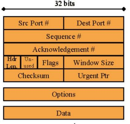
16 bit window size gets Cramped with large Bandwidth x delay
