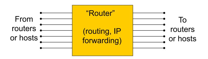
• By convention, draw input ports on left, output on right. (But in reality a single physical port handles both directions.)
