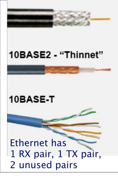
Early types of Ethernet tried to reduce noise purely through shielding
