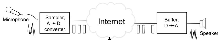
Variable bandwidth and delay (jitter)
