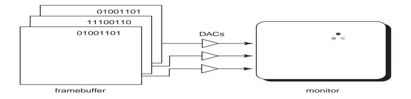
The term **true-color** is sometimes used to refer to systems which the framebuffer directly stores the values of each channel.
