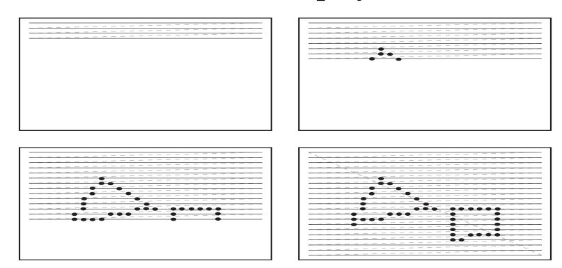
Electron beam traces over screen in raster scan order.
