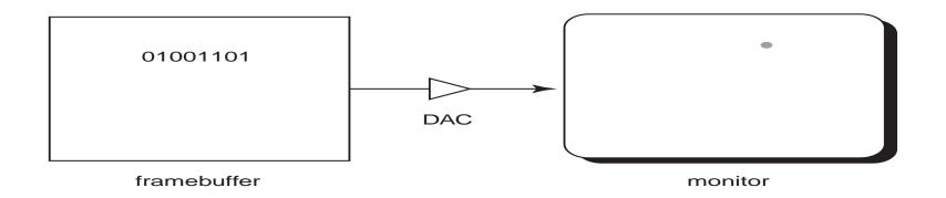
Intensity of the raster scan beam is modulated according to the contents of a **framebuffer**.
