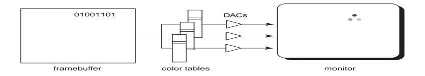
Each framebuffer element is now an index into the color table, where the actual values of each channel are stored.
