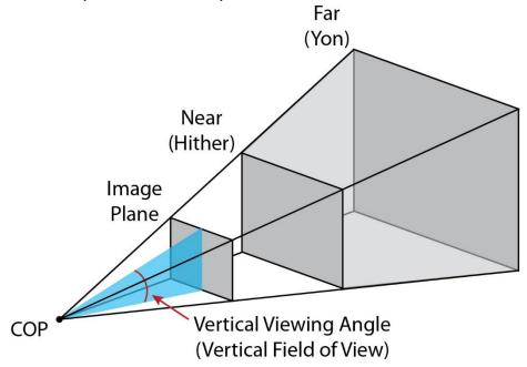
The center of projection and the (finite) image form an infinite pyramid. Objects outside the pyramid are not drawn. The sides of the pyramid are **clipping planes**.
