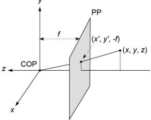
The distance f is called the **focal length** of the pinhole camera , as it is essentially equivalent to the focal length of a lens system in a camera.
