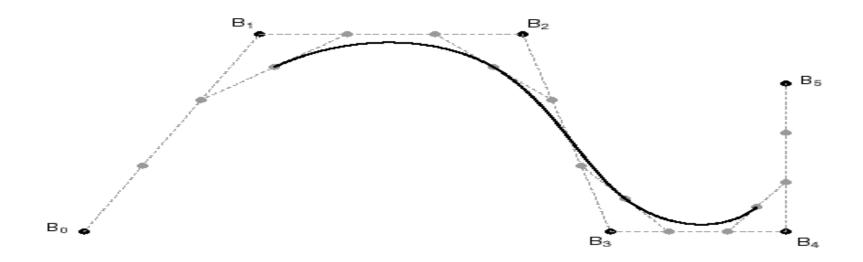
These are called **B-splines**. The starting set of points are called **de Boor points**.
