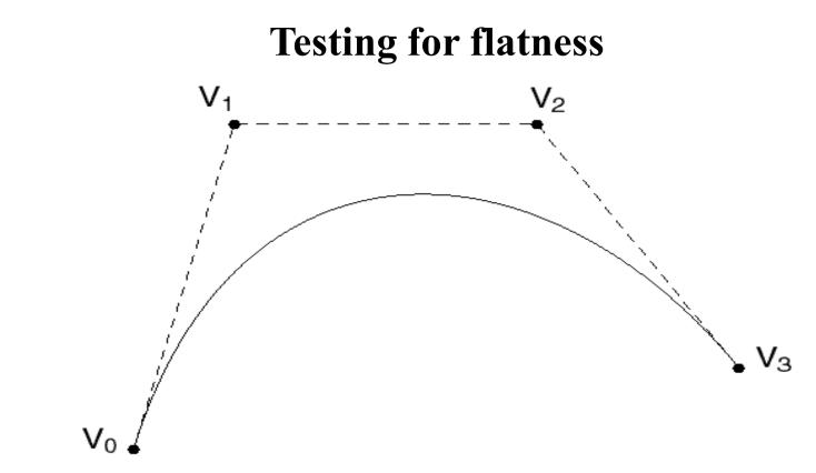
Compare total length of control polygon to length of line connecting endpoints:
