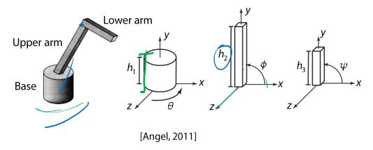
(Note that the angles are set to zero in the figures on the right; i.e., the parts are shown in their "default" positions.)
