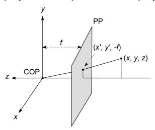
The distance f is called the **focal length** of the pinhole camera , as it is essentially equivalent to the focal length of a lens system in a camera.
