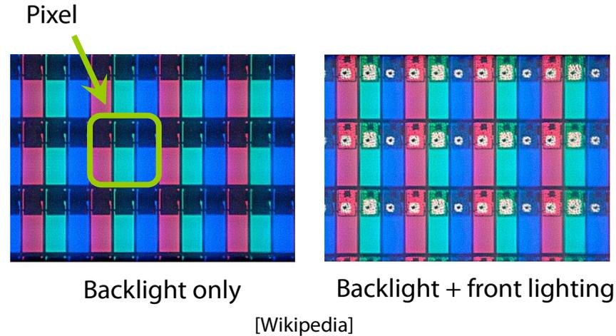
Pixel is one region on the display corresponding to one color sample of an image being shown.
