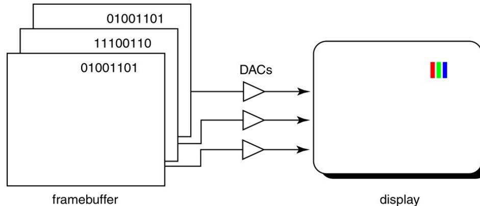
Typically, a display allows 256 voltage settings for each of R, G, and B.
