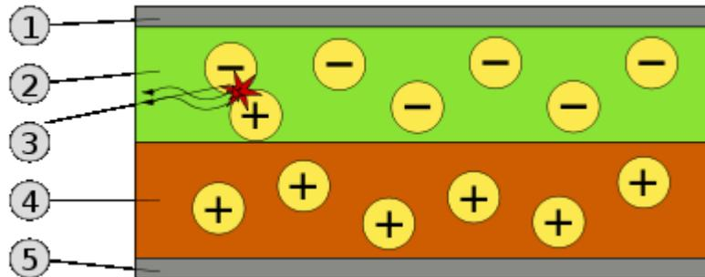
Schematic of a bilayer OLED: 1. Cathode (-), 2. Emissive Layer, 3. Emission of radiation, 4. Conductive Layer, 5. Anode (+). [Wikipedia]
