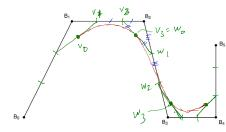
These are called **B-splines**. The starting set of points are called **de Boor points**.
