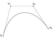
Compare total length of control polygon to length of line connecting endpoints:
