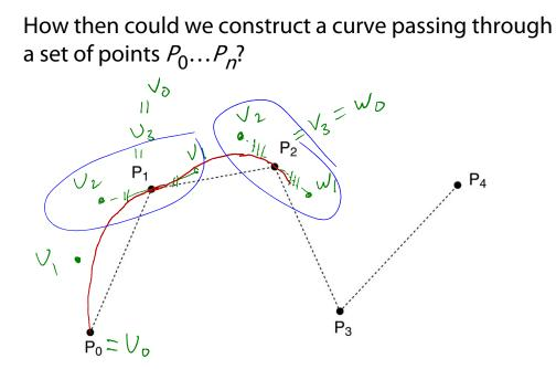
We can specify the Bezier control points directly, or we can devise a scheme for placing them automatically...
