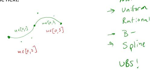
The *u*-range affects placement of control points. The result is a **non-uniform** spline.
