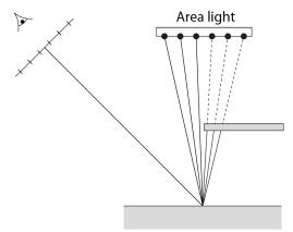
We can trace a ray from the viewer through a pixel, but now when we hit a surface, we cast rays to samples on the area light source.
