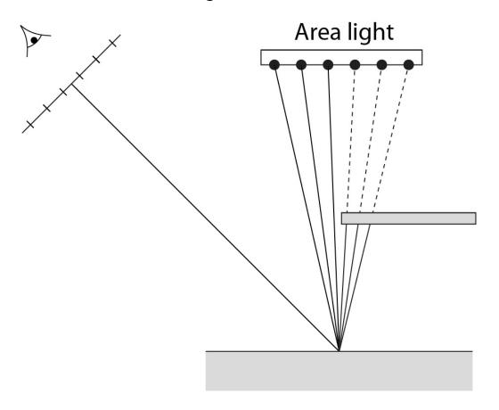
We can trace a ray from the viewer through a pixel, but now when we hit a surface, we cast rays to samples on the area light source.
