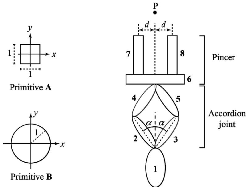
Assume that  $\alpha$  can take values in the range  $[0, 90^\circ]$ . As part of your solution to this problem, you will need to define the instance transformations that should be applied to a given primitive on the left so that it is the same shape as a desired primitive on the right; all scale factors will be integers (1, 2, 3, ...) or simple fractions ( $1/2$ ,  $1/3$ ,  $1/4$ , ...); use a ruler to determine scale factors. Transformations available to you:
