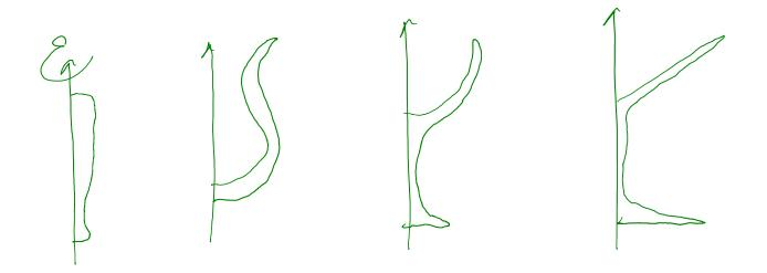
Idea: rotate a 2D **profile curve** around an axis.
