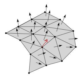
For surfaces of revolution, we can get better-looking results by analytically computing the normal at each vertex...
