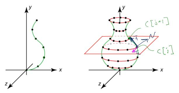
We can compute tangents to the curve points in the *xy*-plane:
