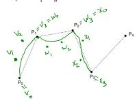
We call this curve a **spline**. The endpoints of the Bezier segments are called **joints**. All other Bezier points (i.e., not endpoints) are called **inner Bezier points**; these points are generally not interpolated.
