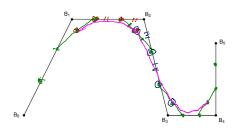
These are called **B-splines**. The starting set of points are called **de Boor points**.
