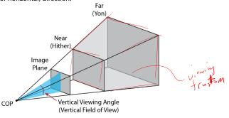
The center of projection and the (finite) image form an infinite pyramid. Objects outside the pyramid are not drawn. The sides of the pyramid are **clipping planes**.
