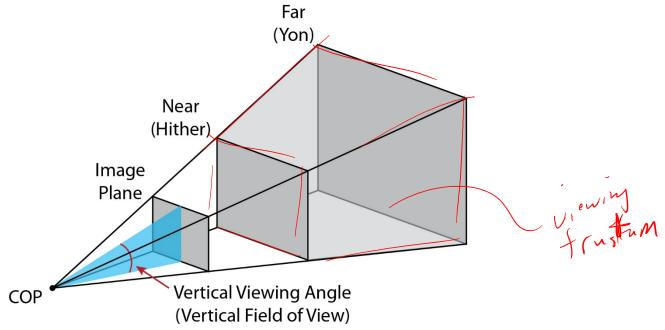
The center of projection and the (finite) image form an infinite pyramid. Objects outside the pyramid are not drawn. The sides of the pyramid are **clipping planes**.
