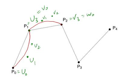
We call this curve a **spline**. The endpoints of the Bezier segments are called **joints**. All other Bezier points (i.e., not endpoints) are called **inner Bezier points**; these points are generally not interpolated.
