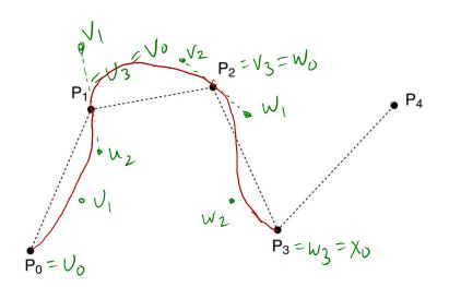
We can specify the Bezier control points directly, or we can devise a scheme for placing them automatically...
