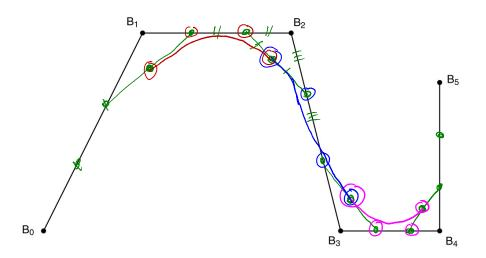
These are called **B-splines**. The starting set of points are called **de Boor points**.
