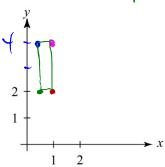
$$\begin{bmatrix} 1/2 & 0 \\ 0 & 2 \end{bmatrix} \qquad \begin{array}{c} \text{Non-uniform sade} \\ \text{a } \neq d \\ \text{x'} = 1/2 \times \\ \text{y'} = 2 \times \\ \end{array}$$
