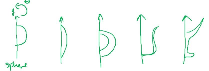
Idea: rotate a 2D **profile curve** around an axis.
