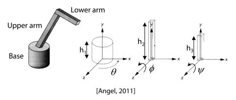
(Note that the angles are set to zero in the figure; i.e., the parts are shown in their "default" positions.)
