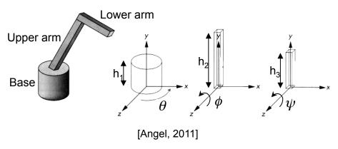
(Note that the angles are set to zero in the figure; i.e., the parts are shown in their "default" positions.)
