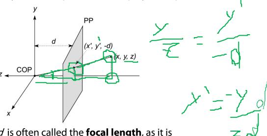
The distance *d* is often called the **focal length**, as it is essentially equivalent to the focal length of a lens system in a camera.
