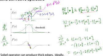
The Sobel operator can produce thick edges. Ideally, we're looking for infinitely thin boundaries.
