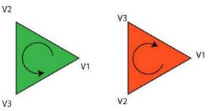
The triangle on the left has a CCW winding order so it will be visible on the screen. The triangle on the right has a CW winding order so you will not see it render on the screen.
