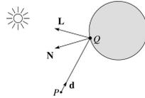
A ray is defined by an origin  $P$  and a unit direction  $\mathbf{d}$  and is parameterized by  $t > 0$ :
