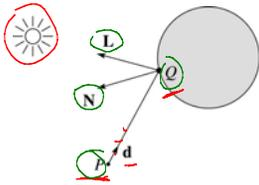
A ray is defined by an origin  $P$  and a unit direction  $\mathbf{d}$  and is parameterized by  $t > 0$ :
