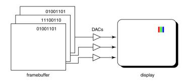
Typically, a display allows 256 voltage settings for each of R, G, and B.
