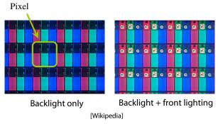
Pixel is one region on the display corresponding to one color sample of an image being shown.
