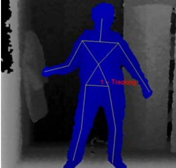
Standard skeleton display (in real time) from PrimeSense, inventor of the Kinect.
