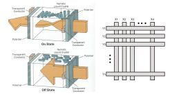
Laptops typically use **liquid crystal displays** (LCD's).
