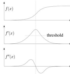
The Sobel operator can produce thick edges. Ideally, we're looking for infinitely thin boundaries.
