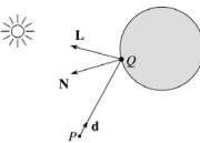
A ray is defined by an origin *P* and a unit direction **d** and is parameterized by t > 0:
