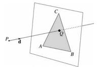
To intersect with a triangle, we first solve for the equation of its supporting plane.
