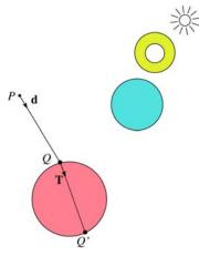
We'll take the view that the color is really only at the surface, like a glass object with a colored transparency coating on it. In this case, we multiply in the transparency constant,  $k_t$ , every time an object is entered or exited, possibly more than once for the same object.
