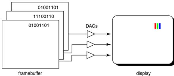
A display that allows 256 voltage settings for each of R, G, and B is known as a **full-color system**
