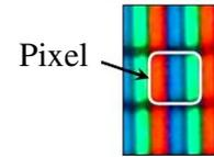
Pixel is one region on the display corresponding to one color sample of an image being shown.
