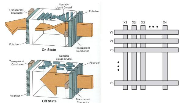
Laptops typically use **liquid crystal displays (LCD's)**.
