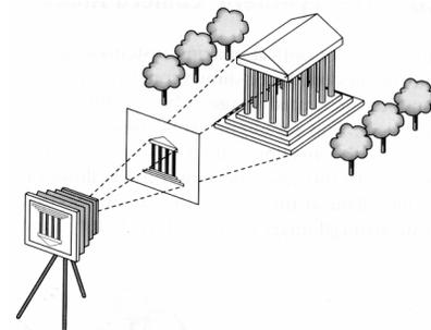
The image is rendered onto an **image plane** (usually in front of the camera).
