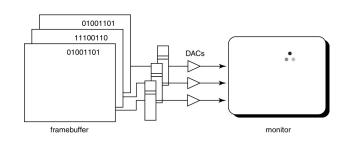
The term **true-color** is sometimes used to refer to systems which the framebuffer directly stores the values of each channel.
