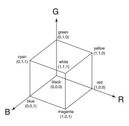
All colors on a monitor or LCD are produced using combinations of red, green, and blue.
