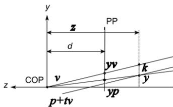
$$y_v = (y+k) \frac{d}{z} \quad \text{and} \quad y_p = y \frac{d}{z}$$
