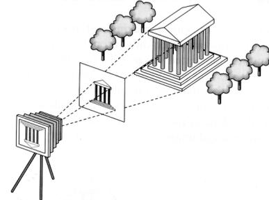
The image is rendered onto an **image plane** (usually in front of the camera).
