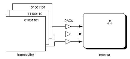
The term **true-color** is sometimes used to refer to systems which the framebuffer directly stores the values of each channel.
