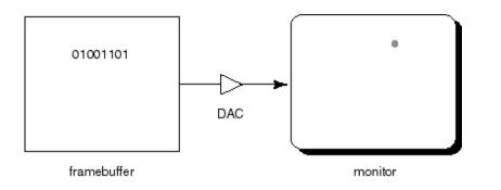
Intensity of the raster scan beam is modulated according to the contents of a **framebuffer**.
