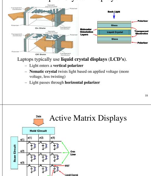
•Active matrix displays have a transistor at each cell. They use a faster switching crystal and transistors that hold charge Passive matrix displays use a matrix of electrodes to control and prevent overflow.
