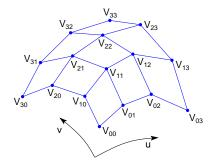
Given a grid of control points  $V_{ii}$ , forming a **control net**, construct a surface S(u,v) by:
