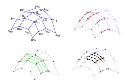
• Which B-spline control points are interpolated by the surface?
