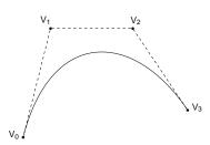
Compare total length of control polygon to length of line connecting endpoints:
