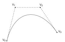
$$Q''(0) = 6(V_0 - 2V_1 + V_2)$$
