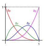
Each Bezier curve is actually a weighted average of four curves: b1, b2, b3, and b4
