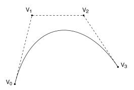
Compare total length of control polygon to length of line connecting endpoints:
