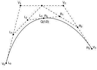
DisplayBezier( V0, V1, V2, V3 ) begin if ( FlatEnough( V0, V1, V2, V3 ) ) Line( V0, V3 ); else Subdivide(V[])  $\Rightarrow$  L[], R[] DisplayBezier( L0, L1, L2, L3 ); DisplayBezier( R0, R1, R2, R3 ); end;
