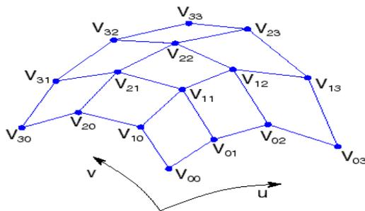
Given a grid of control points  $V_{ij}$  forming a **control net**, construct a surface  $S(u,v)$  by:
