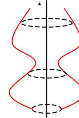
Idea: rotate a 2D **profile curve** around an axis.
