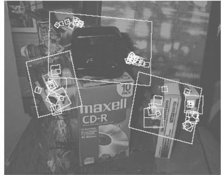
Figure 12: The training images for two objects are shown on the left. These can be recognized in a cluttered image with extensive occlusion, shown in the middle. The results of recognition are shown on the right. A parallelogram is drawn around each recognized object showing the boundaries of the original training image under the affine transformation solved for during recognition. Smaller squares indicate the keypoints that were used for recognition.
